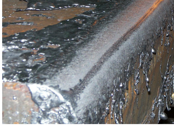
Fig. 3 Slag Coatings after the Scarfing Processing
